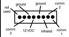
Each RJ45 connector uses 4 wires from MR60 to MVP44a for power, communications and IR. 3 are common, 12VDC, GND (either) and IR. 1 is uniqure 2-way comm (1, 2 or 3) Comm1 goes to keypad slot A1 or B1 Comm2 goes to keypad slot A2 or B2 Comm3 goes to keypad slot A3 or B3
